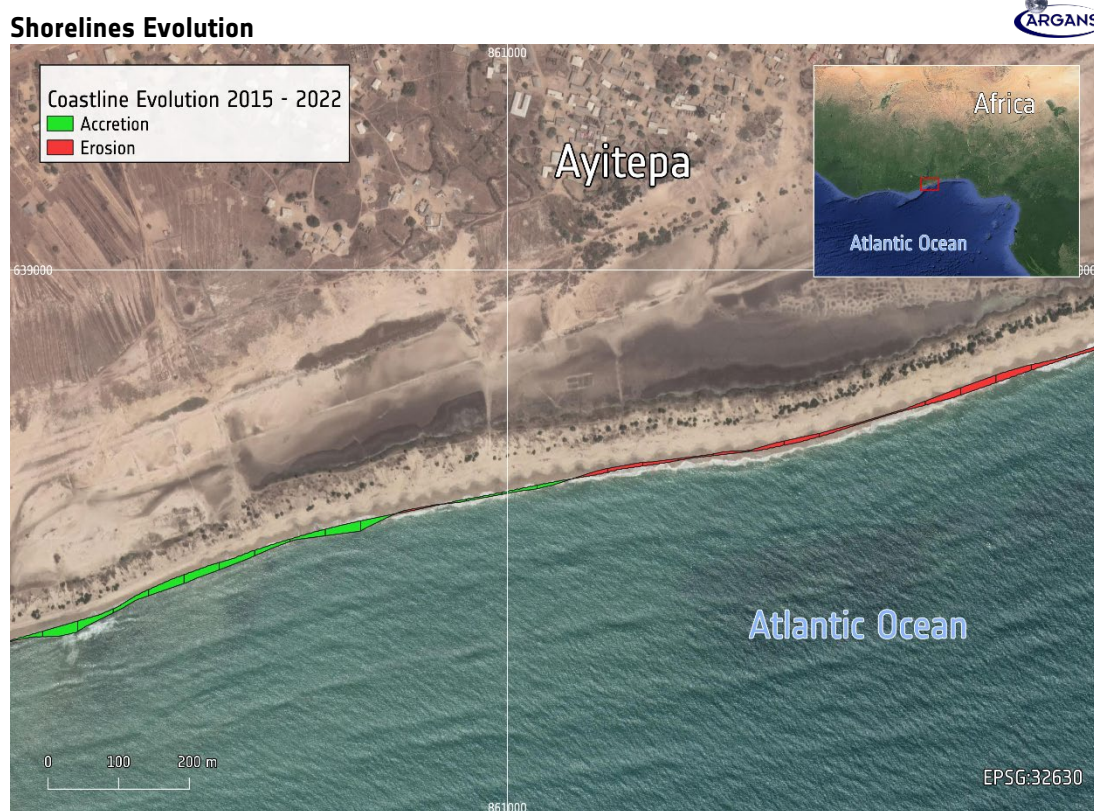
The shoreline evolution map (2013-2022) of Old Ningo, Ghana, illustrates coastline changes, highlighting areas of accretion and erosion. This vital data aids in identifying vulnerable zones,
