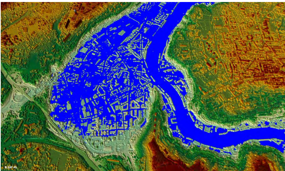
FIGURE 4: 50 cm Multi-Stereo DSM of Lyon, France © 2018, GAF AG, includes EUSI / Maxar material
