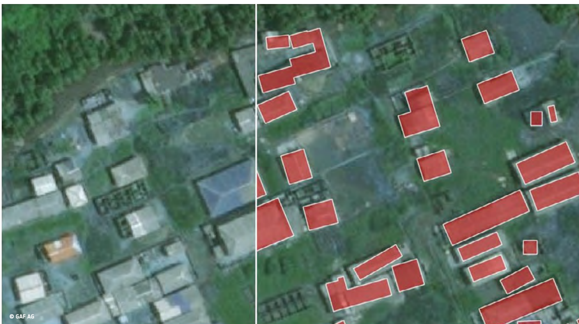
FIGURE 3: AI-derived 2D Building Footprints (R) over Maxar DynamicMosaic (L) in Nigeria © GAF AG
